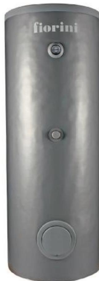
*Water heater for domestic hot water production with single fixed heat exchanger and very thick high-density rigid polyurethane insulation, external metal-coloured PVC coating, magnesium anode for protection against galvanic currents, inspection flange and safety valve.*
