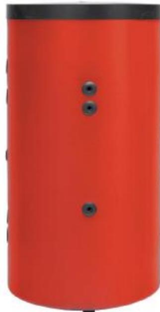
*Water heater for domestic hot water production with single fixed heat exchanger and very thick high-density polyurethane insulation, external PVC coating, magnesium anode for protection against galvanic currents, inspection flange and safety valve.*
