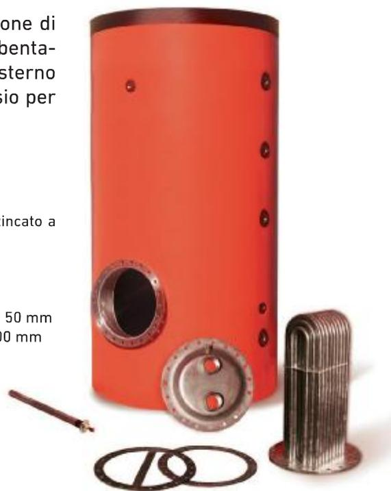
*Water heater with tube bundle heat exchanger for domestic hot water production complete with very thick insulation, external red PVC coating, magnesium anode for protection against galvanic currents.*
