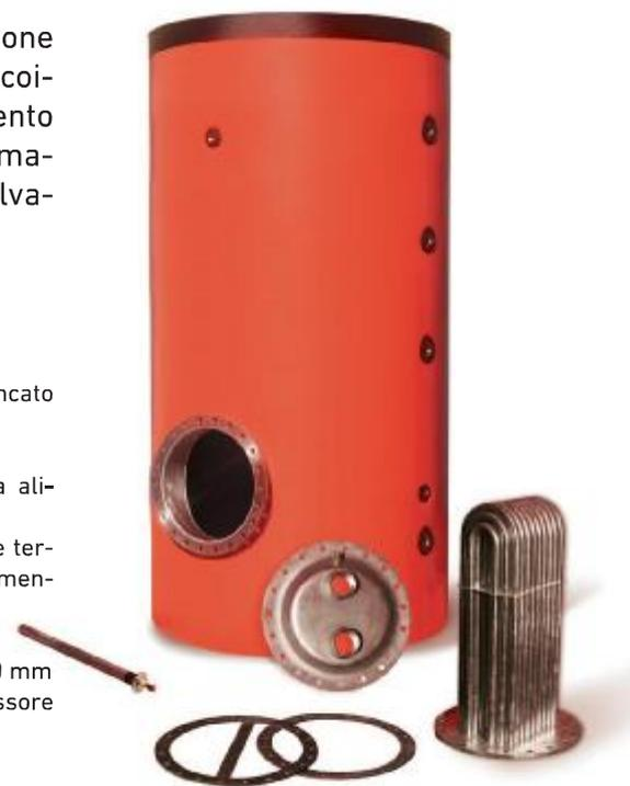
*Water heater with tube bundle heat exchanger for domestic hot water production complete with very thick insulation, external red PVC coating, magnesium anode for protection against galvanic currents.*
